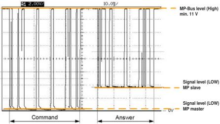
MP-Bus levels OK: Signal level >11 V
